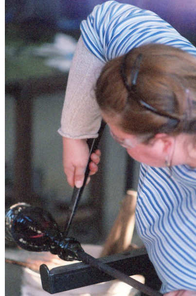
Beth Herbert performing one of the critical points in glassblowing-releasing the piece from the pipe with a few drops of water.
