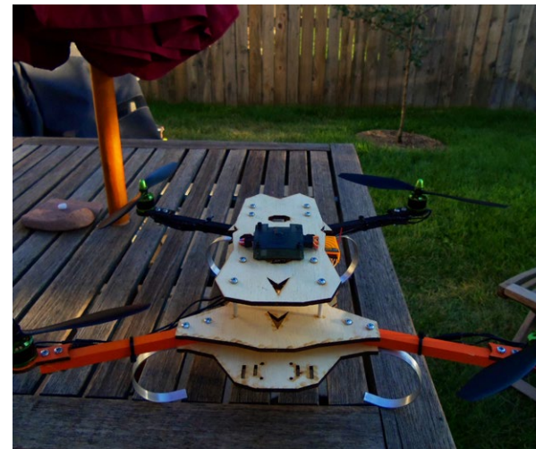
Exploring different materials, this copter was designed in 2D CAD and lasercut out of plywood. It suffered many of the same problems as Lemorange and was almost uncontrollable in flight.
