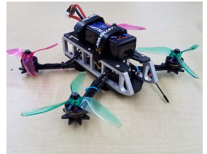
My final prototype for the search and rescue project was machined out of carbon fiber and aerospace aluminum for a rugged, crash-proof drone that had a range of 10 miles.
