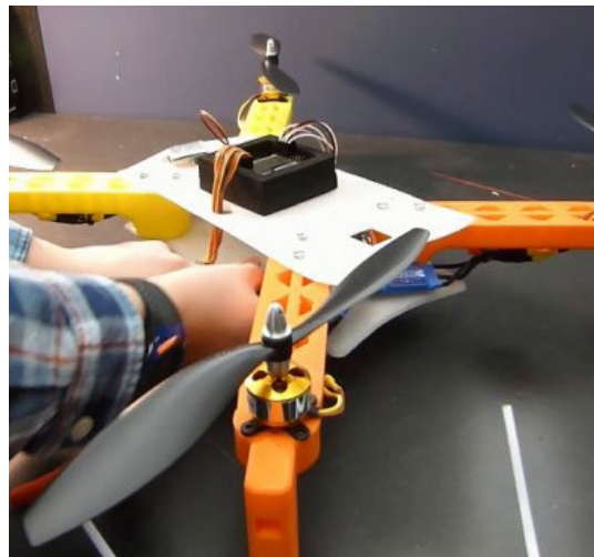
My first design in a middle school club, the "Lemorange" for its yellow and orange 3D-printed arms, had massive 10 inch props spinning on model airplane motors to lift this heavy goliath.
